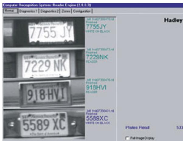
...and send the images to computers that isolate license plates and use machine vision algorithms to read the plate numbers. Once a plate has passed both cameras, the car's travel time is computed.
